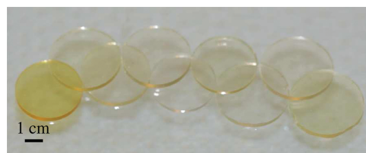
Figure 4. Cut and polished monolithic hybrid silica glasses of approximately 2.5 cm diameter and a thickness of 1 mm.
